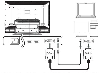
For VGA input, Acer recommends setting your PC's external monitor resolution to 1920 x 1080 pixels @ 30 Hz refresh rate.
